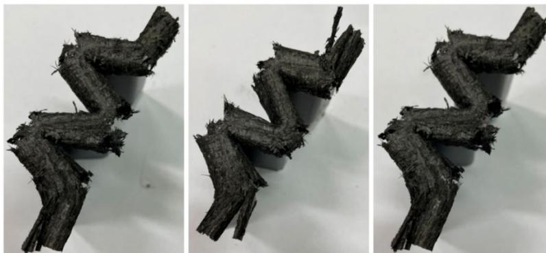
Fig. 1 Impact damage of three repeated W-shaped composite structures
